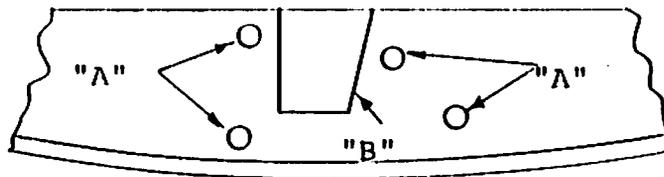
Drill holes "A" using a 1/8" drill. Make sure you drill on the centre of the holes marked on the shell. Countersink the holes to suit the 1 1/4" long 1/4" U.N.F. screws provided. Finally drill 1/4" diameter.
