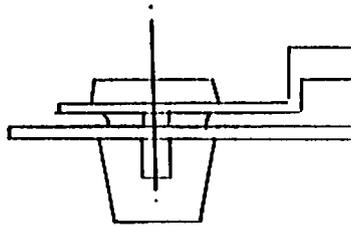
The retaining clip fitted to the slotted operating lever on the latch should be fitted as shown below.
