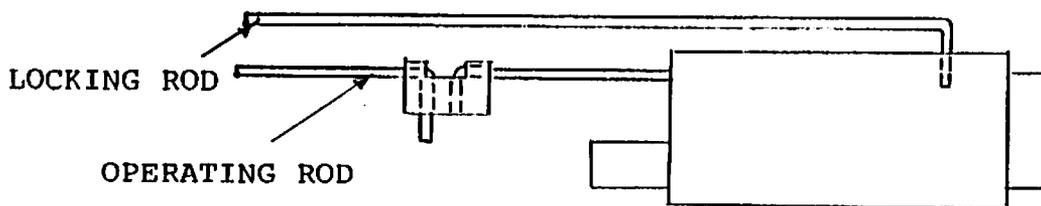
Replace the inner panel over the outer shell and use 2 pop rivets to locate. Lifting edge "A" and looking in direction "A" mark rods. Remove bend and fit clips. Check operation of doors. Secure inner panel to outer shell using 10 No. 1/8" diameter, 1/2" long aluminium pop rivets.
