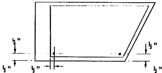
Fit the 2 rods (1 R.H.) into the inner door handle as shown below:-
